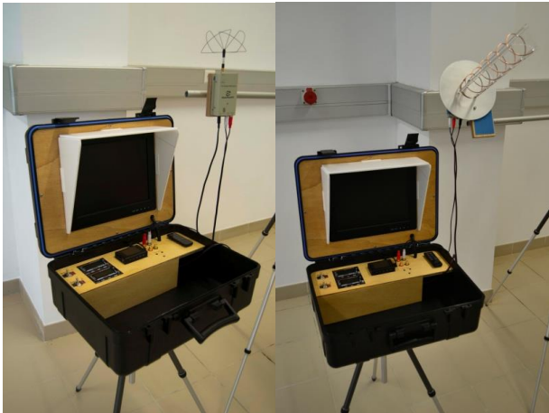
Fig. 24. Complete ground control station showing the video receiver connected to: left) skew planar wheel antenna and right) heliaxial high directivity antenna.
