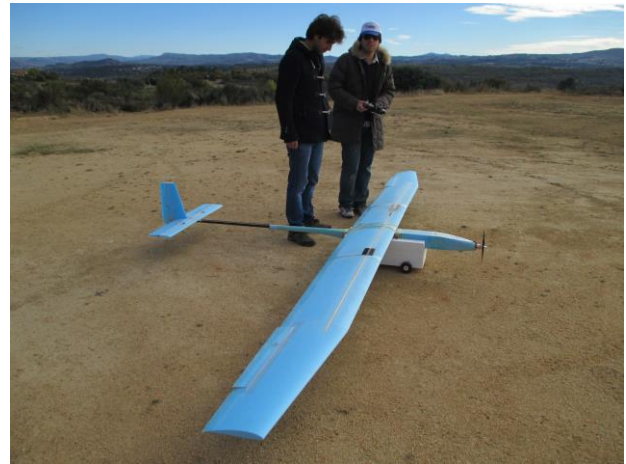
Fig. 28. Initial prototype standing on the buggy and ready for takeoff.
