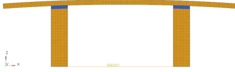
Figure 3: Bumper with the Heat Affected Zone (blue) and unchanged properties (yellow)
