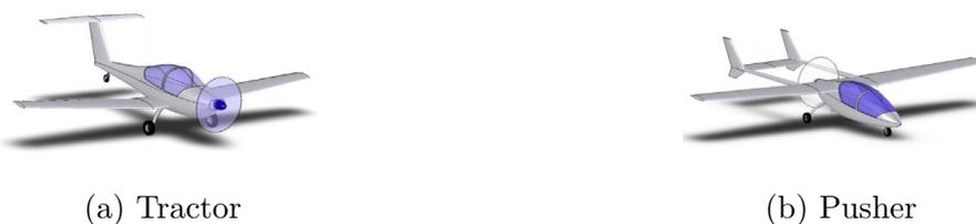
Figure 3: Forward propulsion system configurations [11].
