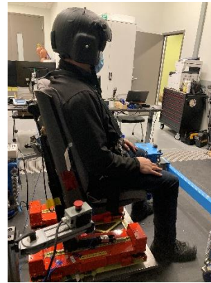
b. active seat mount tested on shaker table
