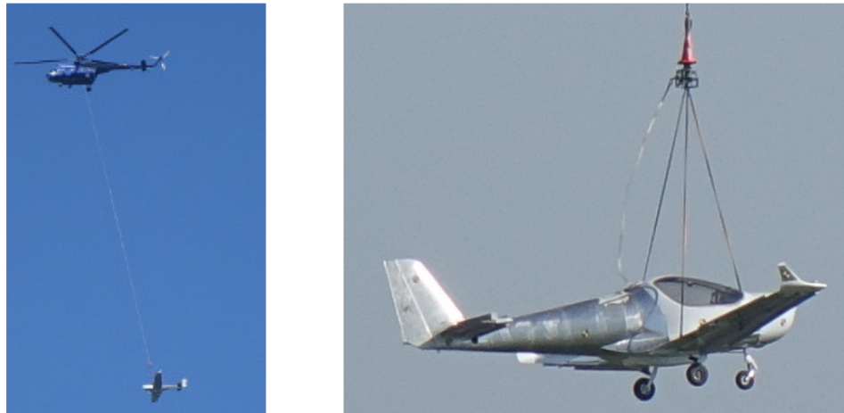
Figure 8. View of the aircraft equipped with the Softland system during a flight test
