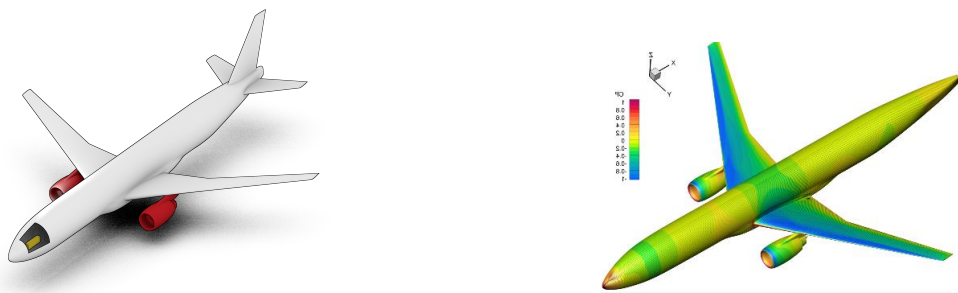
(a) Engines and OBS are highlighted. (b) CFD simulation of nacelle location effects.
