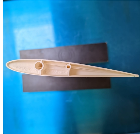
(b) Airfoil and internal structure.
