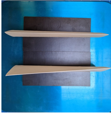
(a) Printed wings with and without twist.
