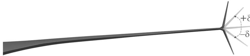
Figure 2: Active winglet principle with variable cant angle.
