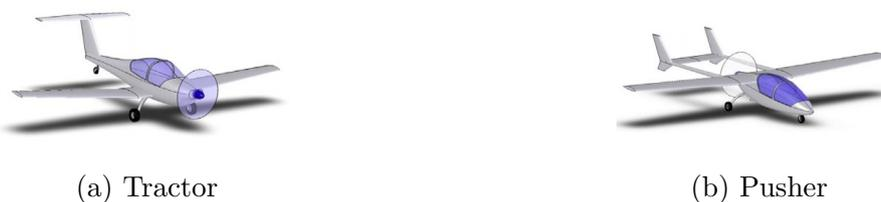
Figure 3: Forward propulsion system configurations [11].
