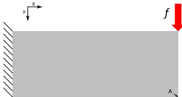
Figure 13: Cantilever beam system where The left boundary is fixed and the force is shown by the red arrow  $f$ . The point at which the displacement will be evaluated is labelled A.
